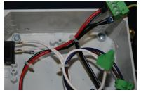
Ensure all three green plugs are properly in place before refitting the lid. Each connection block will only fit one way onto the connector – you won't be able to connect them up incorrectly.
