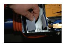
Firmly fasten battery in place and connect the battery lead.
