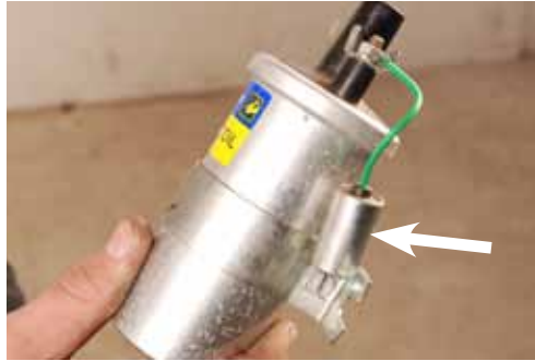
Figure 9. Remove the condenser from the ignition coil.
