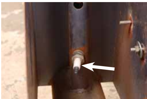
Figure 11. Remove the spark plug to give it a clean.
