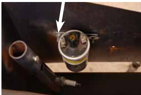
Figure 13. Mount ignition coil back in the chassis. Tighten only the nut furthest away from the barrel for the time being (marked with an arrow).
