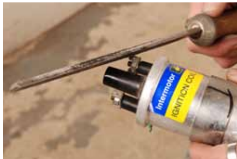
Figure 8. Clean up all the contacts of the ignition coil.
