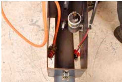
Figure 14. Pass the gas regulator down one side of the barrel and the battery connectors down past the other side of the barrel.
