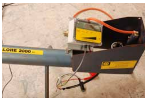
Figure 15. Make sure the control box is the correct way round in the chassis.
