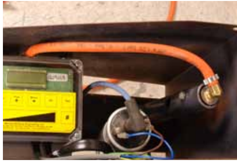
Figure 17. Gently turn the gas injector clockwise in the firing tube so that the gas pipe runs along the wall of the chassis.
