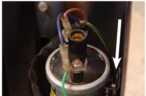
Figure 3. Nut retaining the earth wire from the control box to the coil mounting.
