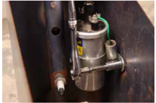
Figure 7. Nut retaining the earth wire from the control box to the coil mounting.
